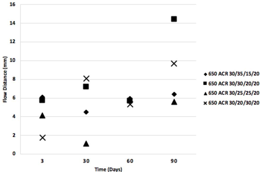
Figure 8. This graph illustrates the distance a constant mass of 650 ACR formulation flowed in 30 seconds as a function of time after the formulation was prepared. The 5 different formulation identities differ by continuous phase ratio of TEGMA and LVM presented as UDMA/TEGMA/LVM/LSM. Each formulation was loaded with 45 w/w% glass, 2 w/w% fumed silica, and 7 w/w% microcapsules.
