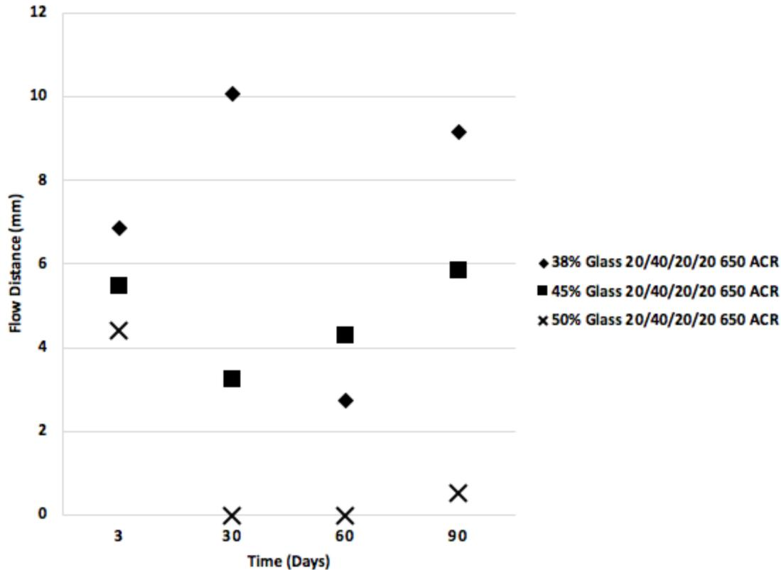
Figure 19. This graph illustrates the distance a constant mass of 650 ACR formulation flowed in 30 seconds as a function of time after the formulation was prepared. The 3 different formulation identities differ by w/w% glass loading. Each formulation was loaded with either 38, 45, or 50 w/w% glass. Each formulation contained 2 w/w% fumed silica, and 7 w/w% microcapsules. The continuous phase ratio (UDMA/TEGMA/LVM/LSM) of 20/40/20/20 was used for each formulation.
