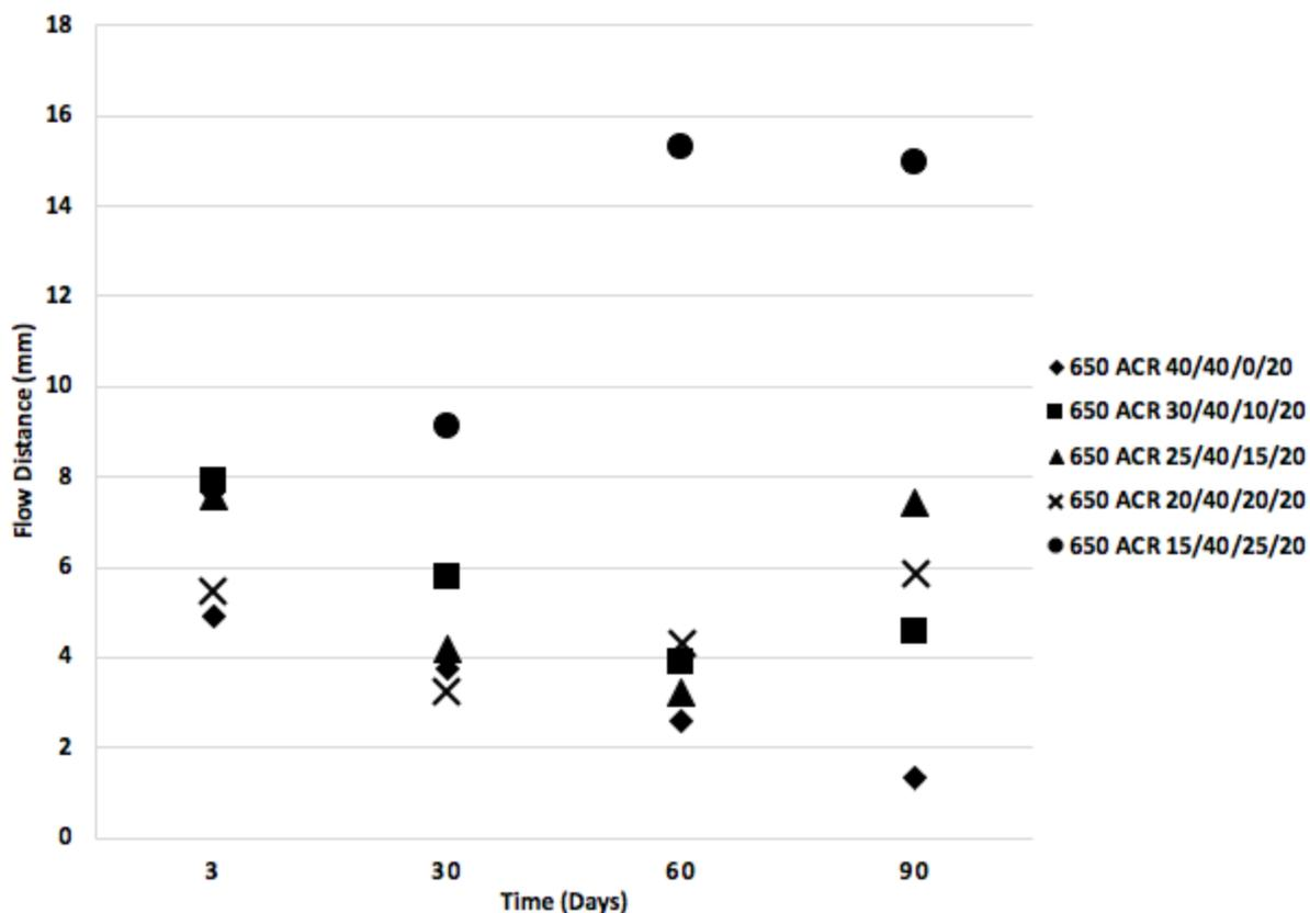
Figure 6. This graph illustrates the distance a constant mass of 650 ACR formulation flowed in 30 seconds as a function of time after the formulation was prepared. The 5 different formulation identities differ by continuous phase ratio of UDMA and LVM presented as UDMA/TEGMA/LVM/LSM. Each formulation was loaded with 45 w/w% glass, 2 w/w% fumed silica, and 7 w/w% microcapsules.
