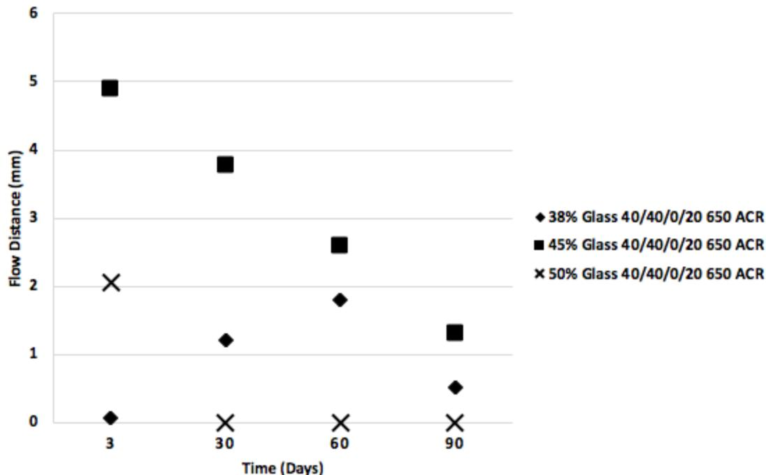
Figure 16. This graph illustrates the distance a constant mass of 650 ACR formulation flowed in 30 seconds as a function of time after the formulation was prepared. The 3 different formulation identities differ by w/w% glass loading. Each formulation was loaded with either 38, 45, or 50 w/w% glass. Each formulation contained 2 w/w% fumed silica, and 7 w/w% microcapsules. The continuous phase ratio (UDMA/TEGMA/LVM/LSM) of 40/40/0/20 was used for each formulation.
