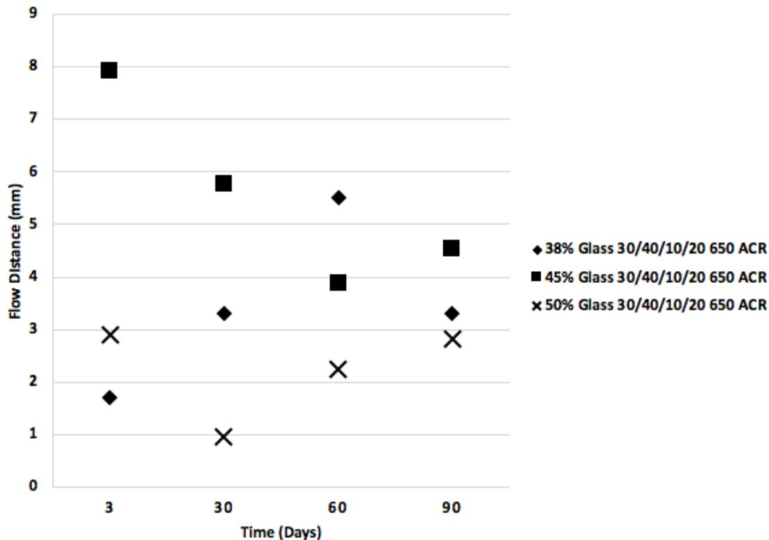
Figure 17. This graph illustrates the distance a constant mass of 650 ACR formulation flowed in 30 seconds as a function of time after the formulation was prepared. The 3 different formulation identities differ by w/w% glass loading. Each formulation was loaded with either 38, 45, or 50 w/w% glass. Each formulation contained 2 w/w% fumed silica, and 7 w/w% microcapsules. The continuous phase ratio (UDMA/TEGMA/LVM/LSM) of 30/40/10/20 was used for each formulation.
