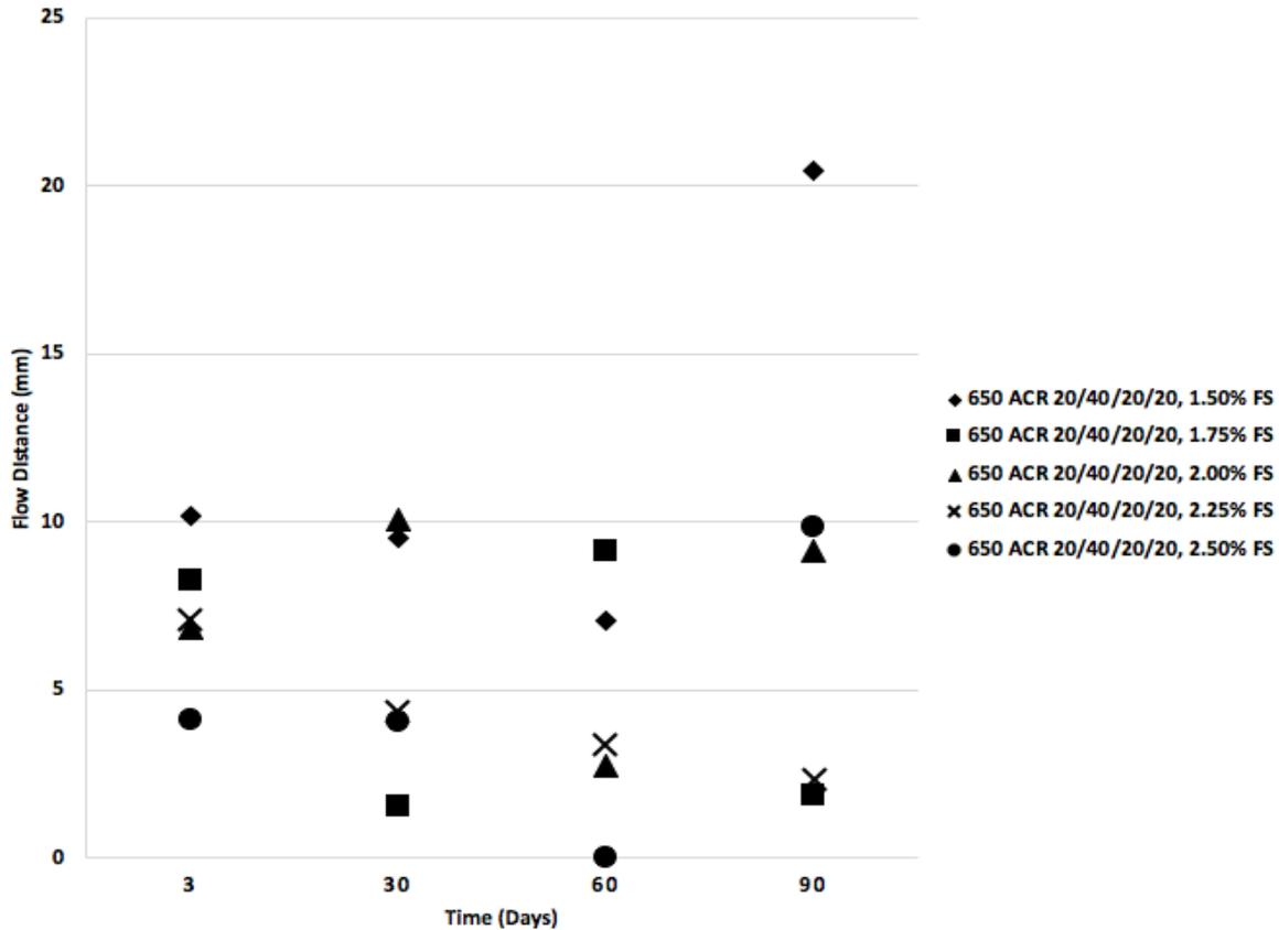
Figure 10. This graph illustrates the distance a constant mass of 650 ACR formulation flowed in 30 seconds as a function of time after the formulation was prepared. The 5 formulations each contain a constant UDMA/TEGMA/LVM/LSM ratio of 20/40/20/20. Each formulation was loaded with 38 w/w% glass, 1.50, 1.75, 2.00, 2.25, or 2.50 w/w% fumed silica, and 7 w/w% microcapsules.
