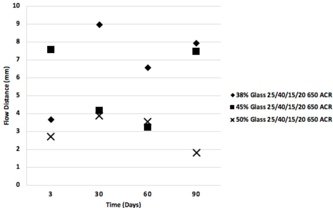
Figure 18. This graph illustrates the distance a constant mass of 650 ACR formulation flowed in 30 seconds as a function of time after the formulation was prepared. The 3 different formulation identities differ by w/w% glass loading. Each formulation was loaded with either 38, 45, or 50 w/w% glass. Each formulation contained 2 w/w% fumed silica, and 7 w/w% microcapsules. The continuous phase ratio (UDMA/TEGMA/LVM/LSM) of 25/40/15/20 was used for each formulation.
