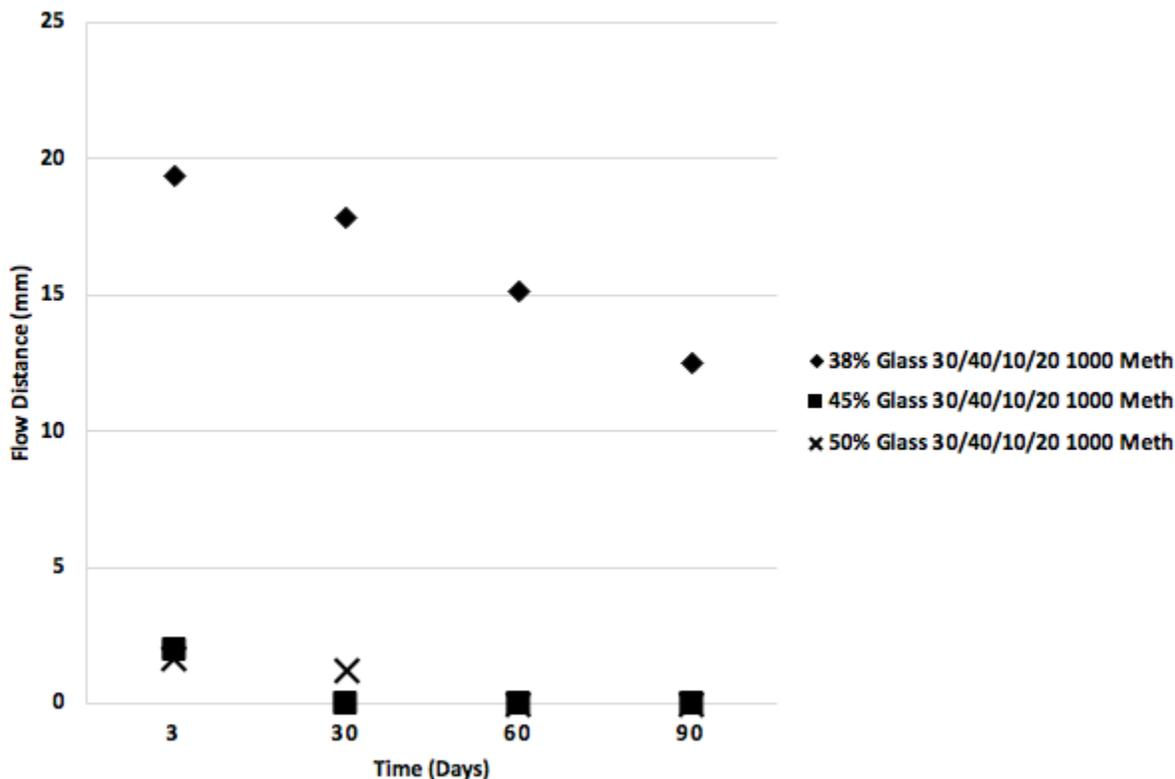
Figure 12. This graph illustrates the distance a constant mass of 1000 Meth formulation flowed in 30 seconds as a function of time after the formulation was prepared. The 3 different formulation identities differ by w/w% glass loading. Each formulation was loaded with either 38, 45, or 50 w/w% glass. Each formulation contained 2 w/w% fumed silica, and 7 w/w% microcapsules. The continuous phase ratio (UDMA/TEGMA/LVM/LSM) of 30/40/10/20 was used for each formulation.
