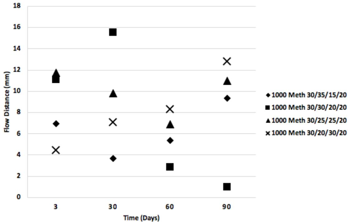
Figure 3. This graph illustrates the distance a constant mass of 1000 Meth formulation flowed in 30 seconds as a function of time after the formulation was prepared. The 5 different formulation identities differ by continuous phase ratio of TEGMA and LVM presented as UDMA/TEGMA/LVM/LSM. Each formulation was loaded with 38 w/w% glass, 2 w/w% fumed silica, and 7 w/w% microcapsules.
