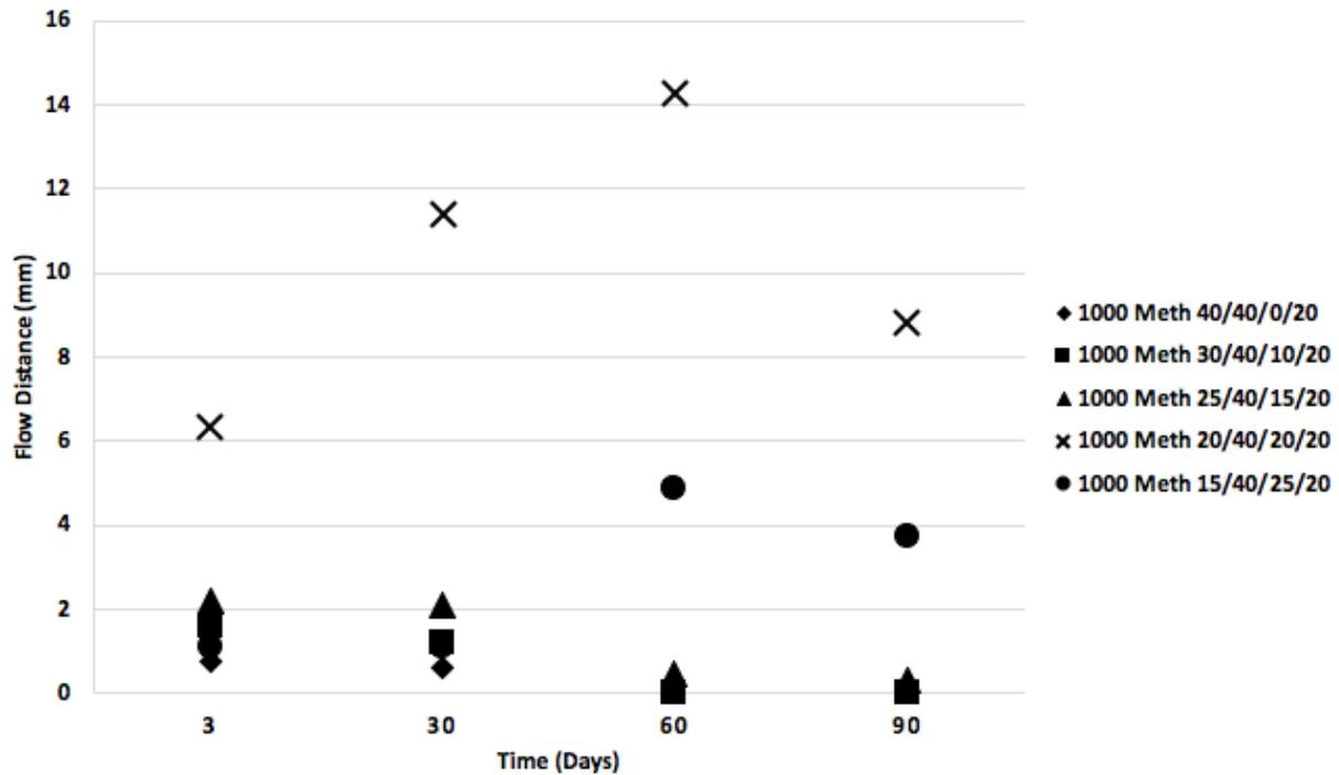
Figure 4. This graph illustrates the distance a constant mass of 1000 Meth formulation flowed in 30 seconds as a function of time after the formulation was prepared. The 5 different formulation identities differ by continuous phase ratio of UDMA and LVM presented as UDMA/TEGMA/LVM/LSM. Each formulation was loaded with 50 w/w% glass, 2 w/w% fumed silica, and 7 w/w% microcapsules.
