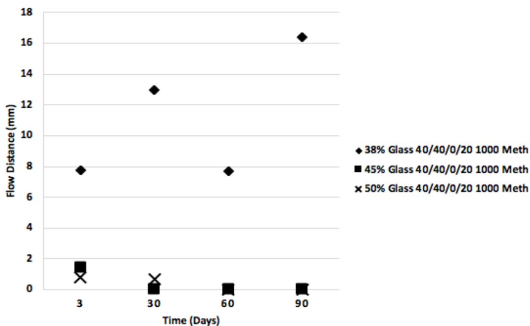
Figure 11. This graph illustrates the distance a constant mass of 1000 Meth flowed in 30 seconds as a function of time after the formulation was prepared. The 3 different formulation identities differ by w/w% glass loading Each formulation was loaded with either 38, 45, or 50 w/w% glass. Each formulation contained 2 w/w% fumed silica, and 7 w/w% microcapsules. The continuous phase ratio (UDMA/TEGMA/LVM/LSM) of 40/40/0/20 was used for each formulation.
