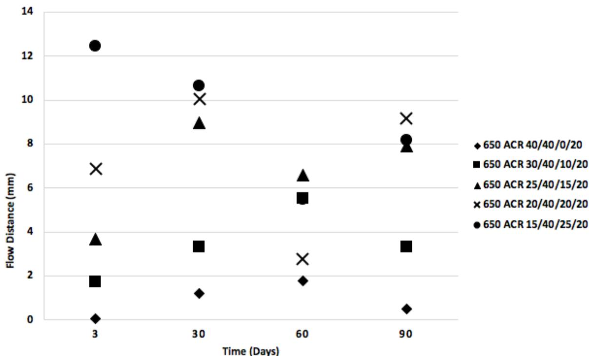
Figure 2. This graph illustrates the distance a constant mass of 650 ACR formulation flowed in 30 seconds as a function of time after the formulation was prepared. The 5 different formulation identities differ by continuous phase ratio of UDMA and LVM presented as UDMA/TEGMA/LVM/LSM. Each formulation was loaded with 38 w/w% glass, 2 w/w% fumed silica, and 7 w/w% microcapsules.
