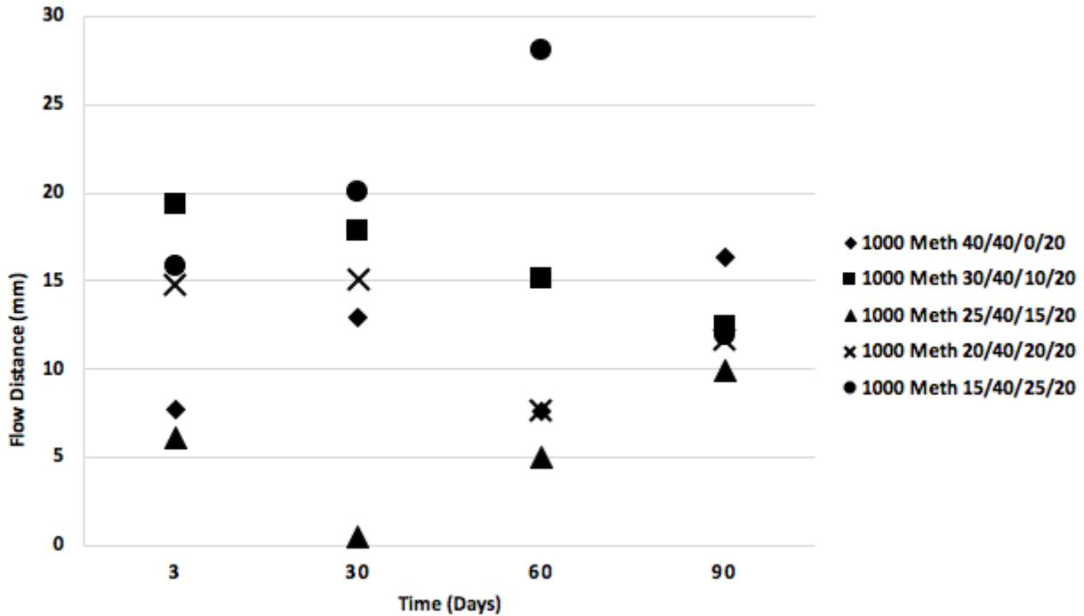
Figure 1. This graph illustrates the distance a constant mass of 1000 Meth formulation flowed in 30 seconds as a function of time after the formulation was prepared. The 5 different formulation identities differ by continuous phase ratio of UDMA and LVM presented as UDMA/TEGMA/LVM/LSM. Each formulation was loaded with 38 w/w% glass, 2 w/w% fumed silica, and 7 w/w% microcapsules.
