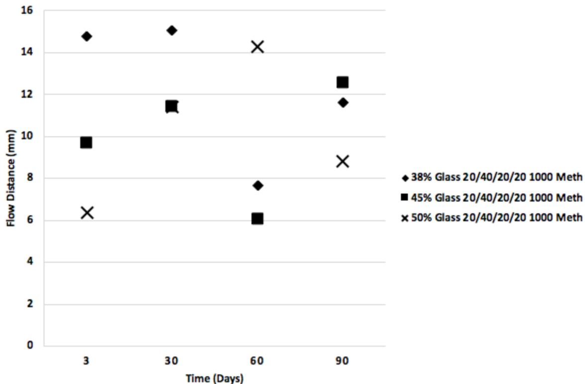
Figure 14. This graph illustrates the distance a constant mass of 1000 Meth flowed in 30 seconds as a function of time after the formulation was prepared. The 3 different formulation identities differ by w/w% glass loading. Each formulation was loaded with either 38, 45, or 50 w/w% glass. Each formulation contained 2 w/w% fumed silica, and 7 w/w% microcapsules. The continuous phase ratio (UDMA/TEGMA/LVM/LSM) of 20/40/20/20 was used for each formulation.
