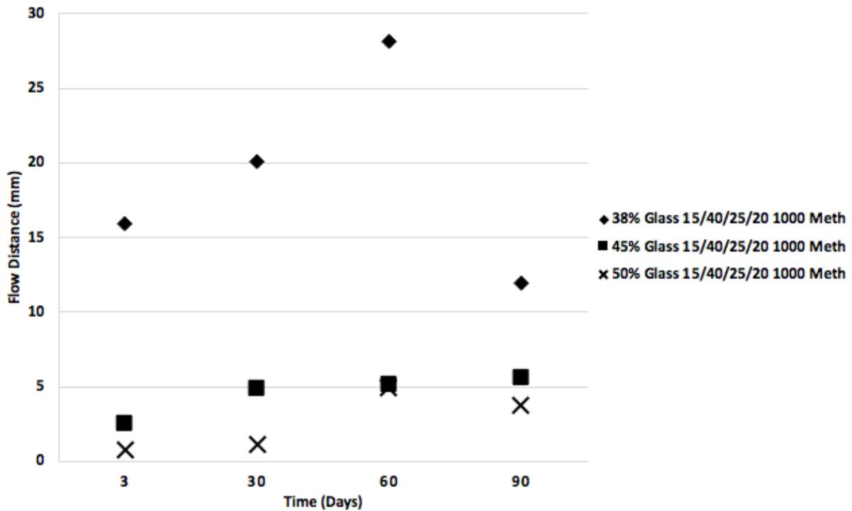
Figure 15. This graph illustrates the distance a constant mass of 1000 Meth formulation flowed in 30 seconds as a function of time after the formulation was prepared. The 3 different formulation identities differ by w/w% glass loading. Each formulation was loaded with either 38, 45, or 50 w/w% glass. Each formulation contained 2 w/w% fumed silica, and 7 w/w% microcapsules. The continuous phase ratio (UDMA/TEGMA/LVM/LSM) of 15/40/25/20 was used for each formulation.
