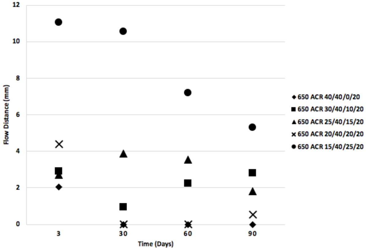
Figure 7. This graph illustrates the distance a constant mass of 650 ACR formulation flowed in 30 seconds as a function of time after the formulation was prepared. The 5 different formulation identities differ by continuous phase ratio of UDMA and LVM presented as UDMA/TEGMA/LVM/LSM. Each formulation was loaded with 50 w/w% glass, 2 w/w% fumed silica, and 7 w/w% microcapsules.
