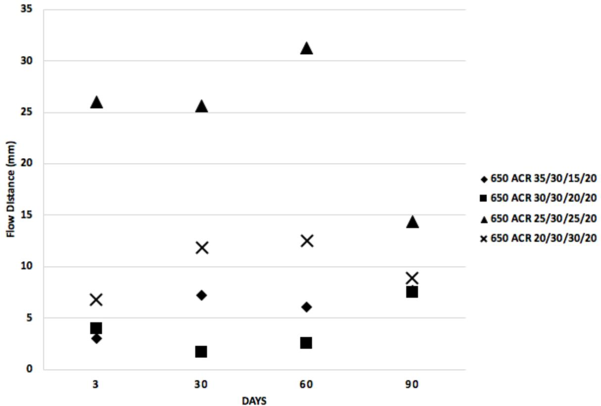
Figure 9. This graph illustrates the distance a constant mass of 650 ACR formulation flowed in 30 seconds as a function of time after the formulation was prepared. The 5 different formulation identities differ by continuous phase ratio of UDMA and LVM presented as UDMA/TEGMA/LVM/LSM. Each formulation was loaded with 38 w/w% glass, 2 w/w% fumed silica, and 7 w/w% microcapsules.
