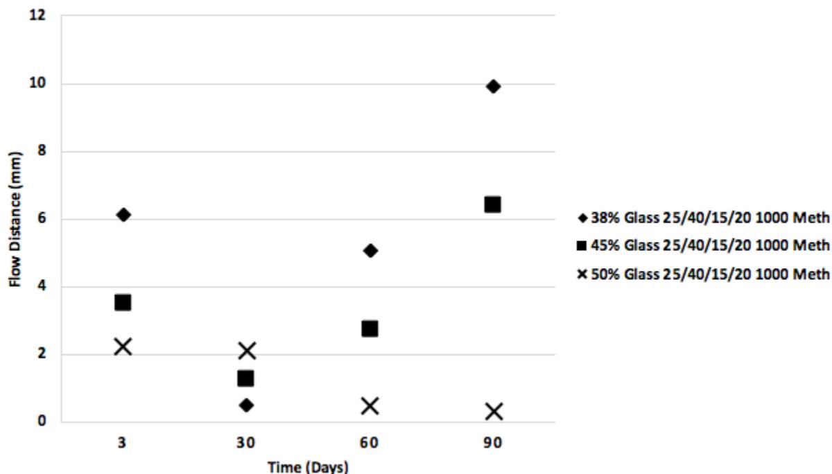
Figure 13. This graph illustrates the distance a constant mass of 1000 Meth formulation flowed in 30 seconds as a function of time after the formulation was prepared. The 3 different formulation identities differ by w/w% glass loading. Each formulation was loaded with either 38, 45, or 50 w/w% glass. Each formulation contained 2 w/w% fumed silica, and 7 w/w% microcapsules. The continuous phase ratio (UDMA/TEGMA/LVM/LSM) of 25/40/15/20 was used for each formulation.
