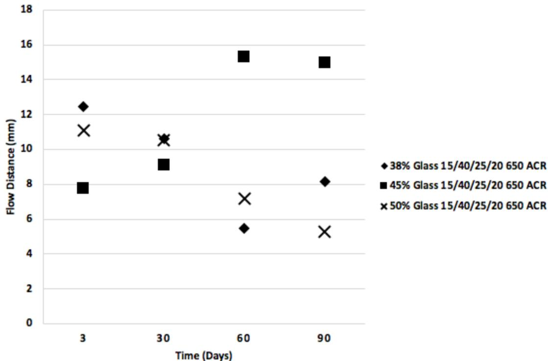
Figure 20. This graph illustrates the distance a constant mass of 650 ACR formulation flowed in 30 seconds as a function of time after the formulation was prepared. The 3 different formulation identities differ by w/w% glass loading. Each formulation was loaded with either 38, 45, or 50 w/w% glass. Each formulation contained 2 w/w% fumed silica, and 7 w/w% microcapsules. The continuous phase ratio (UDMA/TEGMA/LVM/LSM) of 15/40/25/20 was used for each formulation.
