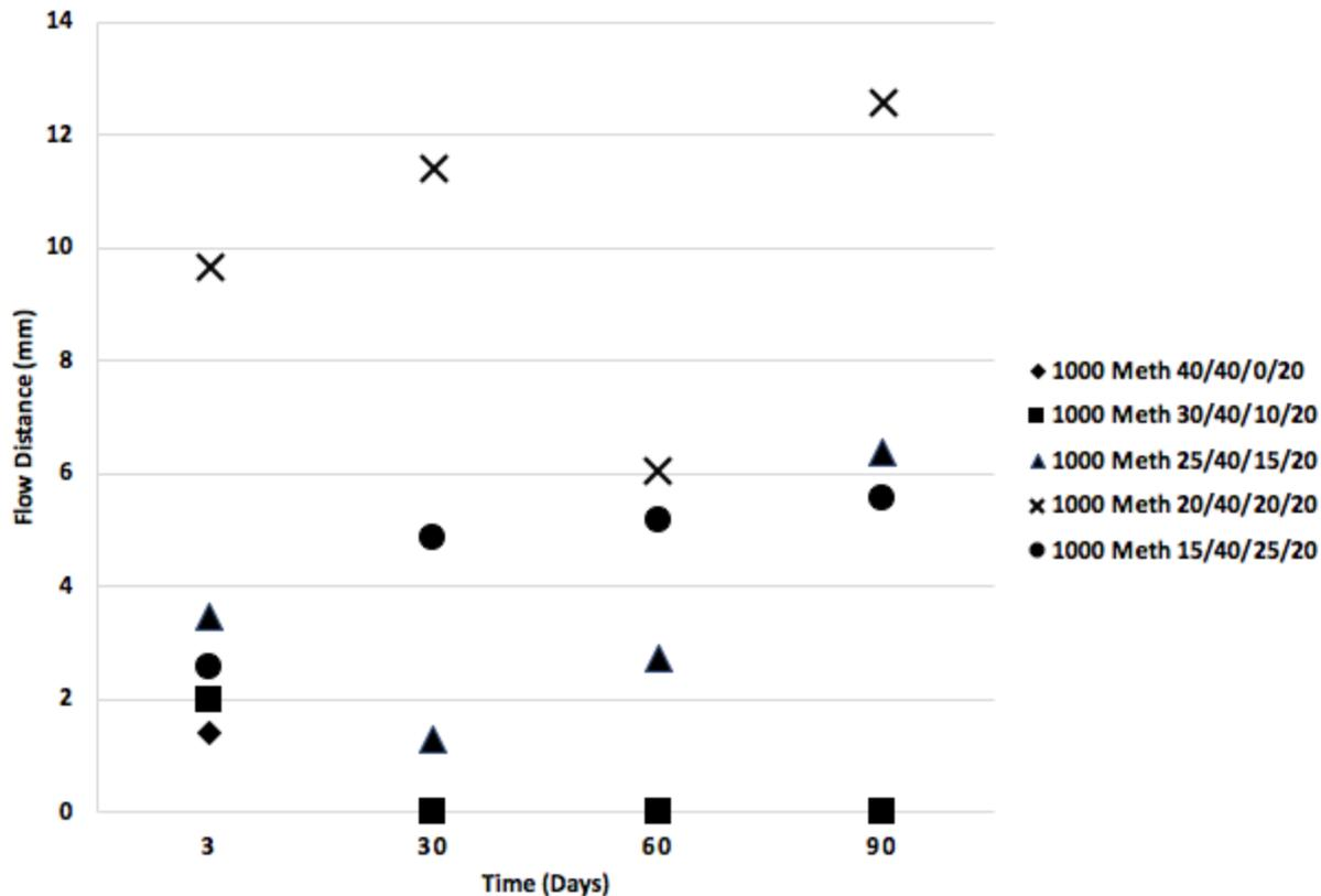
Figure 5. This graph illustrates the distance a constant mass of 1000 Meth formulation flowed in 30 seconds as a function of time after the formulation was prepared. The 5 different formulation identities differ by continuous phase ratio of UDMA and LVM presented as UDMA/TEGMA/LVM/LSM. Each formulation was loaded with 45 w/w% glass, 2 w/w% fumed silica, and 7 w/w% microcapsules.
