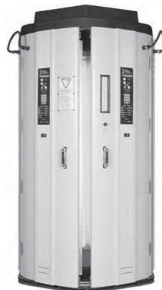
Figure 2: Ultraviolet light box used to provide a specific amount of UVB light.
